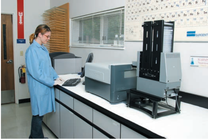
Figure 12. The Odyssey Sa can be configured to work with the optional BioTek® BioStack™ Automated Microplate Stacking system.
